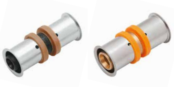
Obr. 50. Spojka KAN-therm ultraPRESS k trubkám PERTAL, PEXC, PERT a blueFLOOR PERT, 14 × 2, 16 × 2, 20 × 2, 25 × 2,5 mm.
